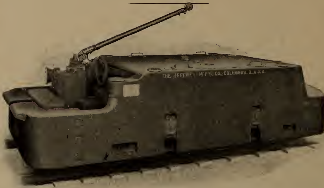
JEFFREY D. M. 105, 13 TON ELECTRIC MINE LOCOMOTIVE. DRAW BAR PULL 5000 POUNDS.
